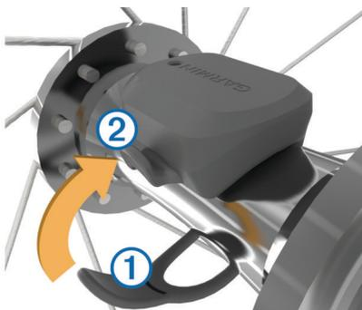
The sensor may be tilted when installed on an asymmetrical hub. This does not affect operation.
