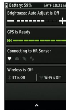
The connections screen appears. A flashing icon means the device is searching. You can select any icon to change the settings.
